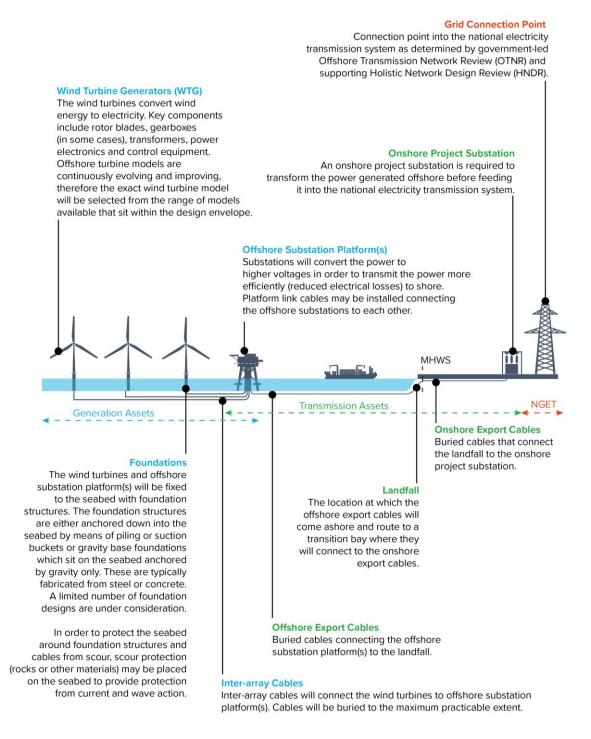
Plate 1.1 Components of Morecambe Offshore Windfarm (generation and transmission). Generation Assets are in blue (included in this ES) and Transmission Assets are in green.
